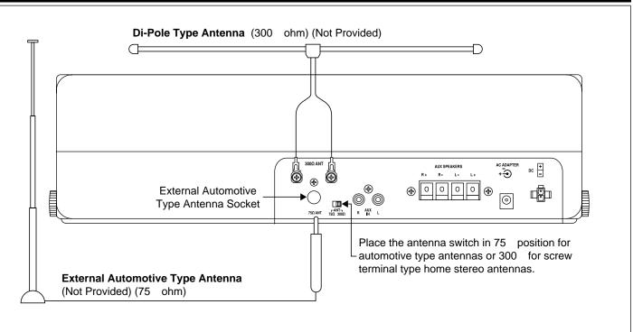
The units will accept either a standard automotive type antenna plug or the screw terminals of a  $300\Omega$  ohm di-pole wire antenna typically used in a home stereo system. Follow the diagram enclosed for the antenna type your are installing
